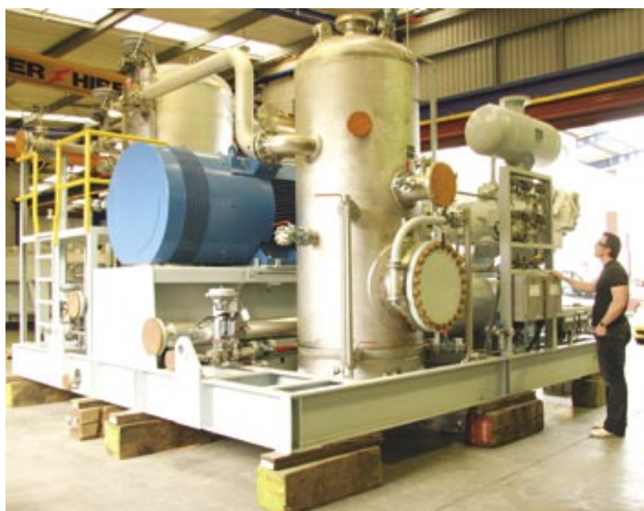
Flash Gas Compressor for the Kupe Gas Project in Taranaki
